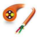
Robust PCF installation cable for assembly (IP20 heads only) for installation in stationary systems and machines, aramid strain relief elements, with individual elements made from FRNC material, halogen-free, ozone and UV resistant, with a polyurethane (PUR) outer sheath
